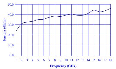
Field strength (dBV/m) = Output measured (dBV) + Antenna Factor (dB/m)
